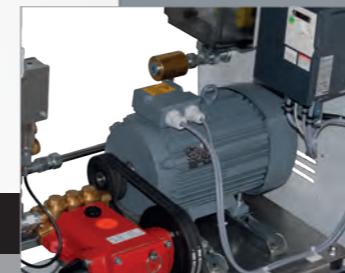
• The carbon dioxide filling unit CFA 3 can accurately and economically fill CO 2 fire extinguishers or CO 2 cylinders up to 50 kg to weight thanks to short set-up times and rapid working speeds. The system has a low rate of wear and is low-maintenance.
