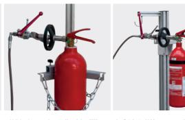
• With the carbon dioxide filling unit CFA 5-2W you can fill CO, fire extinguishers or CO<sub>2</sub> cylinders up to 50 kg.
