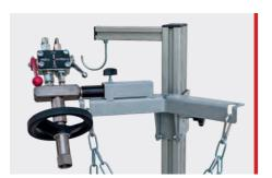
• The filling armature of the CFA 5-2W has one filling and one release ball valve and can be attached to the CO<sub>2</sub> cylinder as well as to the scales platform as necessary.
