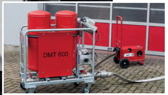
• DMT 600 flow meter in use.
