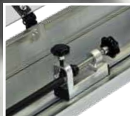
• Testing of a stored pressure fire extinguisher hose which is sealed by the longitudinally flexible nozzle closure of the SPGV.
