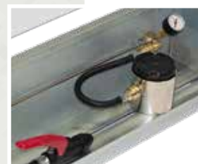
• Testing of a safety valve with a valve testing adapter.
