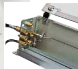
• Testing of a stored pressure fire extinguisher hose which is sealed by the longitudinally flexible nozzle closure of the SPGV.
